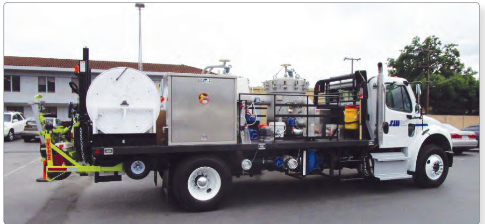
SJWC's new zero-discharge flushing truck cleans water mains more effectively than conventional flushing while conserving water.
